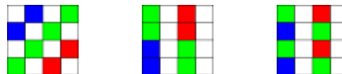
Figure 3-14 : Examples of 4x4 CFA from Kodak using red-green-blue-white pixels (image from Wikipedia)
