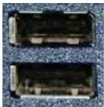
The USB2 ports conform to the USB 2.0 standard. These ports are usually used for USB2 Flash Drives but are also sometimes used for a keyboard and mouse.
