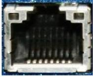
The Gigabit Ethernet port conforms to the IEEE 802.3 1000BASE-T standard for Gigabit Ethernet over copper. We recommend using Category 5e or Category 6 compatible cabling and connectors for best performance.
