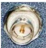
The NTSC/PAL port provides an external camera video signal input that can be synchronized with the higher resolutions LightWise™ IQ camera video stream. This is used to provide context between the higher resolution images and the NTSC/PAL Video Stream running at a higher frame rate (25 fps or 30 fps).
